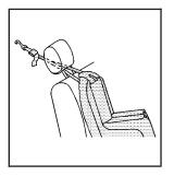
If the position you are using has an adjustable headrest or head restraint and you are using a dual tether, route the tether under the head restraint and in between the head restraint posts.
